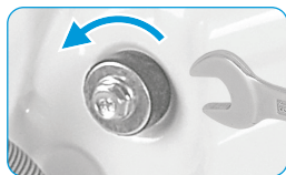
Loosen the 4 transport bolts with a spanner
