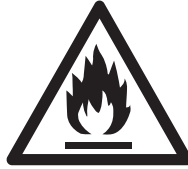
Caution: Risk of fire/ flammable materials
