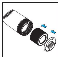
6. Turn the base cover clockwise from **OPEN** position to **LOCK** position, you will hear a "click" sound, the base cover is fastened. (f)
