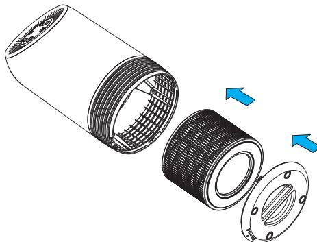
5. Turn the base cover clockwise from **OPEN position** to **LOCK position**. When you hear a "click" sound, the base cover is fastened.
