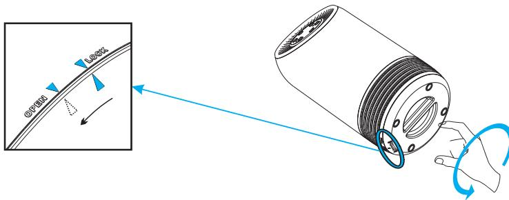
2. Remove the base cover and take out the filter.
