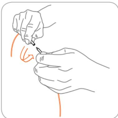
Press until both connectors meet together, and turn it clockwise to fasten it.
