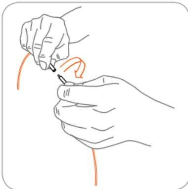
While pressed, turn the connector on the right counterclockwise to remove it.
