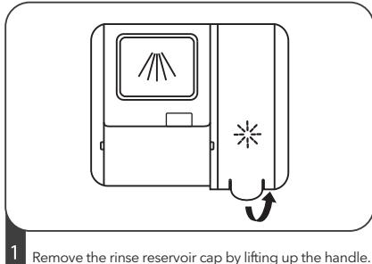
1 Remove the rinse reservoir cap by lifting up the handle.
