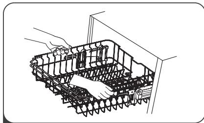
**1** To raise the the upper basket, just lift the upper basket at the center of each side until the basket locks into place in the upper position. It is not necessary to lift the adjuster handle.
