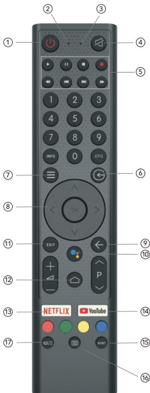
1. Switches the TV between on and standby mode
