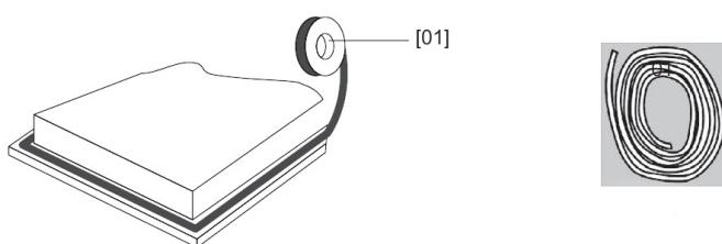
Stretch out the supplied seal along the underside edge of the hob, ensuring the ends overlap.
