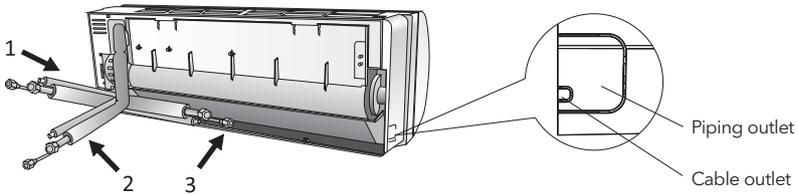
2. Bending the connecting pipes with the port facing up as shown in the figure.
