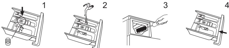
Press the release and remove the dispenser drawer
