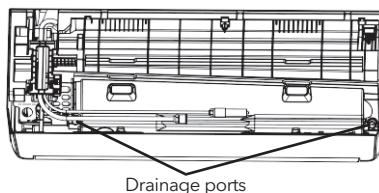
2. Connect the drainage hose to the drainage port, ensure the joint is firm and the sealing effect is good.
