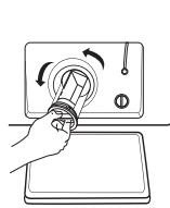
Open the filter by turning to the counter clockwise
