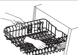
**1** To raise the rack to the upper position, lift rack until both sides are at the same height. The rack will secure into place.
