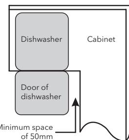
**Step 2. Aesthetic panel's dimensions and installation**
