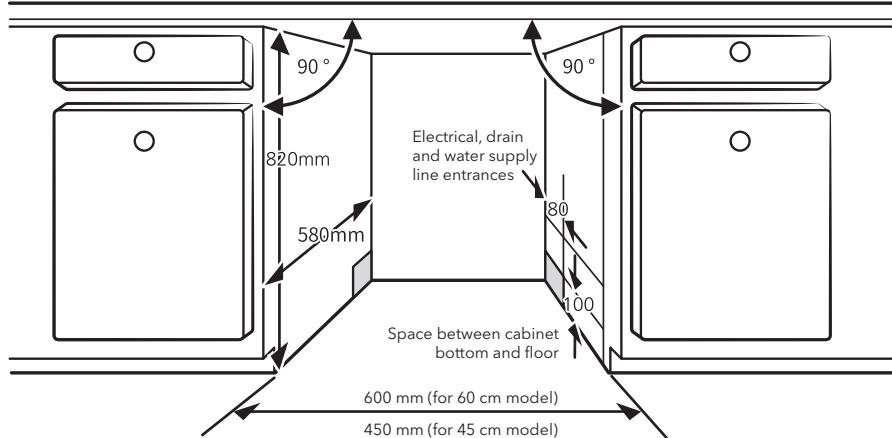
2. If dishwasher is installed at the corner of the cabinet, there should be some space left for when the door is opened.
