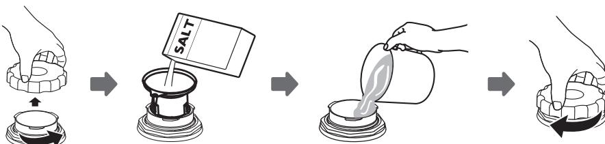
1. Remove the lower basket and unscrew the reservoir cap.
