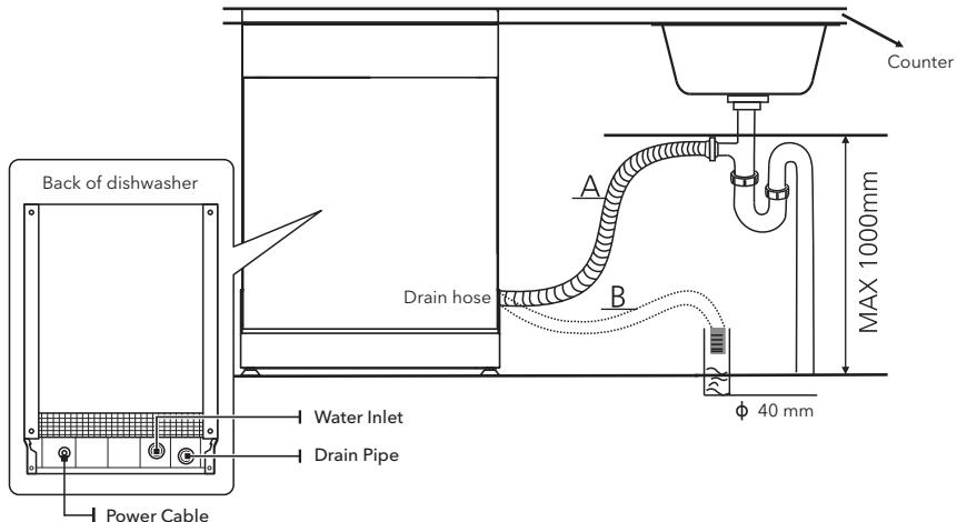
**How to drain excess water from hoses**
