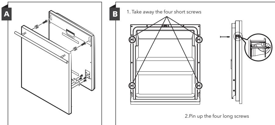
**Step 3. Tension adjustment of the door**
