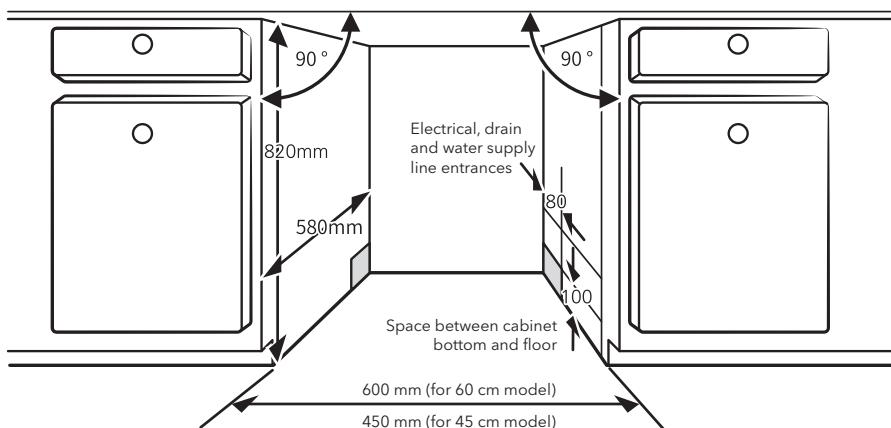
2. If dishwasher is installed at the corner of the cabinet, there should be some space left for when the door is opened.
